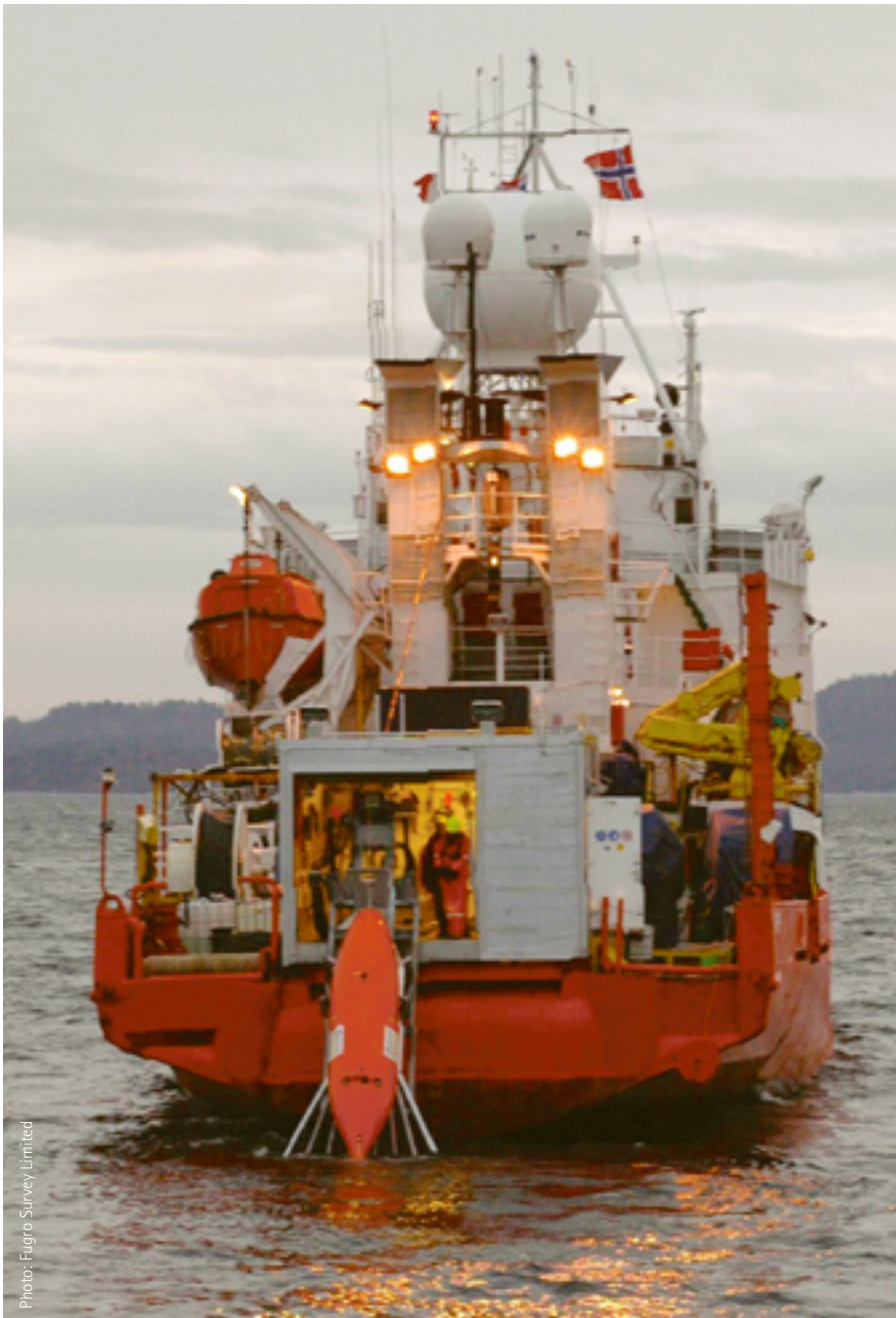
The autonomous underwater vehicle is hauled back on board the Geo Prospector in Norway, having undertaken detailed seabed survey trials at water depths of several hundred metres.
